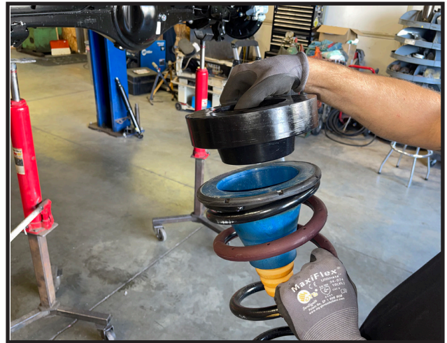
31. Locate the new rear coil spacers and install on the top of the OE rear coils and bump jouncers.
