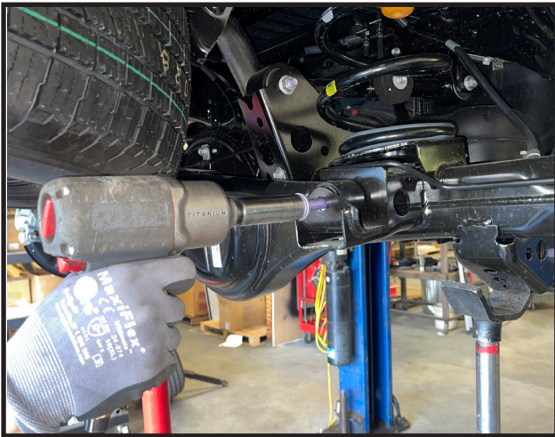
29. On the driver side of the axle housing, locate the ABS sensor wire and remove the mounting hardware from the axle bracket. Save hardware.
