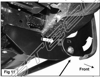
Insert a Plastic Washer between the Grille Guard and the Frame Mounting Bracket on each 12mm Hex Bolt
