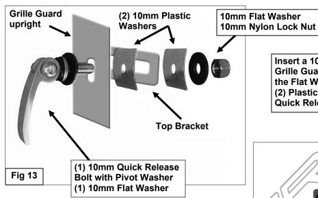
Insert a 10mm Plastic Washer between the Grille Guard and the Top Bracket and under the Flat Washer on each Quick Release Bolt.
