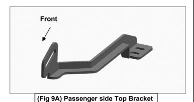
Insert Top Bracket into opening in bumper (Grille guard pictured installed for reference only do not install at this time)
