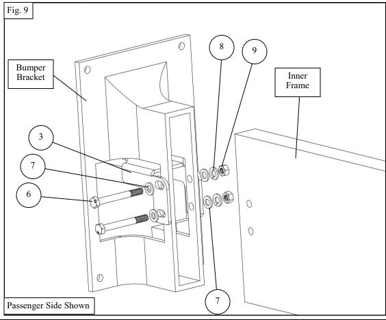
11. With the help of another person or lift, raise the grille guard into place and install to the mounting brackets using the supplied M12 hardware. **See Figure 10-11.**
