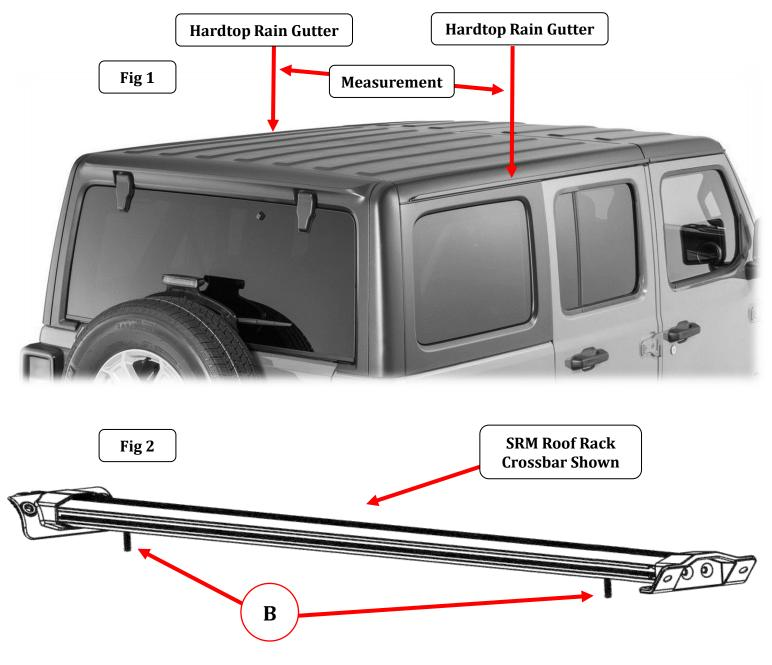
Step-2 Fully assemble the SRM Roof Rack.
