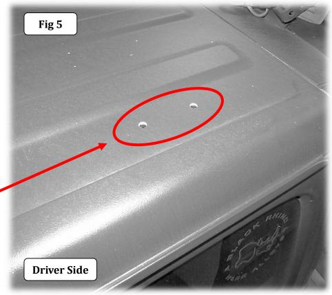
**Step-7** Reinstall the driver side rear bracket using the M8 hex head bolts and M8 washers. Snug but do not tighten the bolts.
