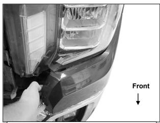
(Fig 3) Pull outward to release plastic fascia body panel from clips. Do not remove, only release inner end to remove grille
