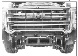
(Fig 20) Tow hooks and all Brackets installed. Reinstall grille and plastic cover
