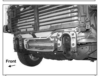
(Fig 9) Remove tow hooks, bumper brackets and shutter assembly if equipped
