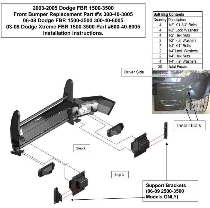
**<u>Step 1:</u>** Remove factory bumper. Note: **<u>Do not</u>** remove factory tow hooks.
