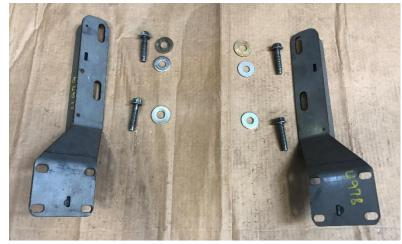
2. Install frame mounts onto the truck frame where the tow hooks were removed. On the rear hole, use one washer between the frame and the mount. Of the remaining washers, use 1 washer per bolt. Do NOT fully tighten.
