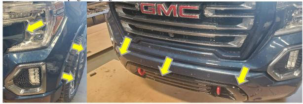
7. Using a 10mm, remove the (3) bolts holding the bottom of the grill in. Unplug the camera on the right side of the grill and remove the grill.
