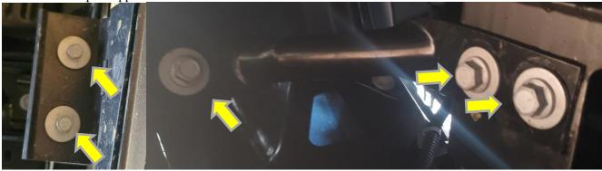
11. Using an 18mm and 10 inch extension, remove (4) bumper bolts from the top of the bumper. Remove
