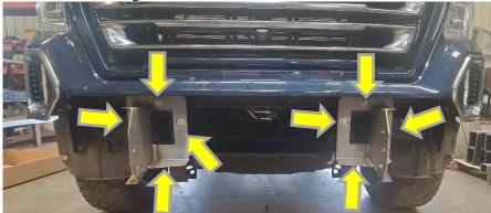
4. Layout hardware from hardware kit #1. Use (6) bolts, (6) flat washers, and (6) flat washers with (2) weld nut tab 3's.
