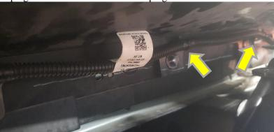
10. Using a 10mm and 15mm, remove (6) bolts from the outer bumper supports and (4) bolts from inner
