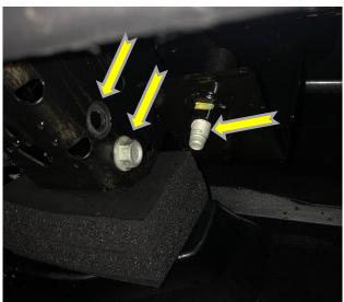
3. Once the tow hook bolts are removed, pull the tow hooks through the front of the bumper to remove them. There are foam blocks between the bumper and the frame that can make this step difficult, but the tow hook will pull through it. Once removed, set the tow hooks, OE hardware, and foam pieces to the side, they will not be used again.
