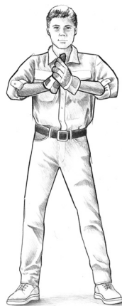
6) Braking Cross your palms together to tell the driver to apply the foot brake.
