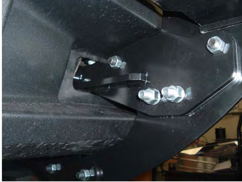
Figure 7. Mounting Side Member.
