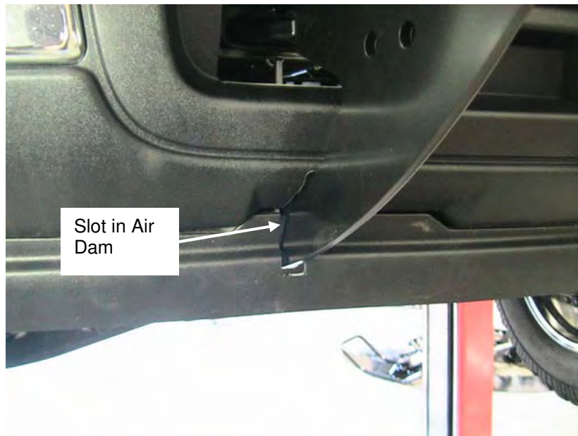
Figure 6. Side Member Through Slot. (GMC Sierra)
