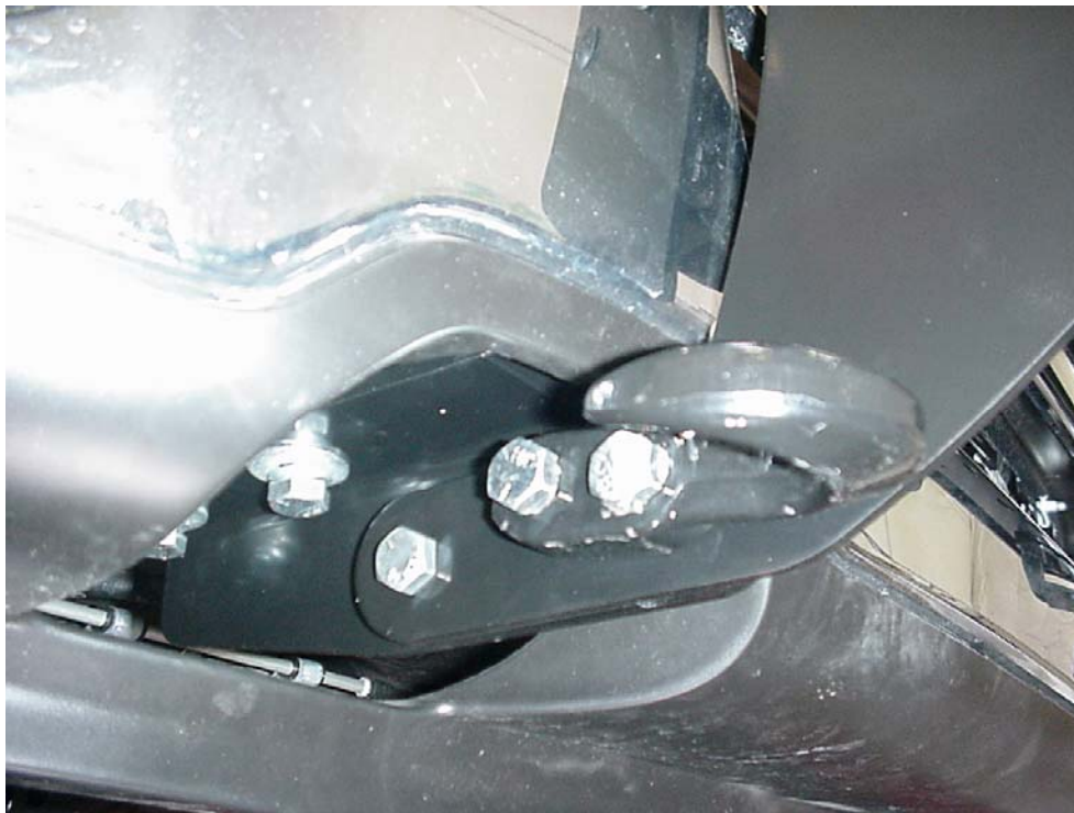
Figure 10 RH Tow Hook, Side Member and Bottom Bracket assembled
