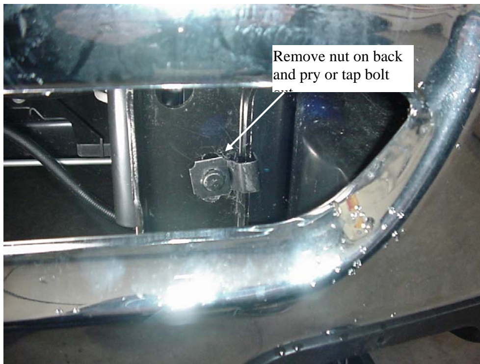
Figure 6 Inboard bumper bolt –left side shown
