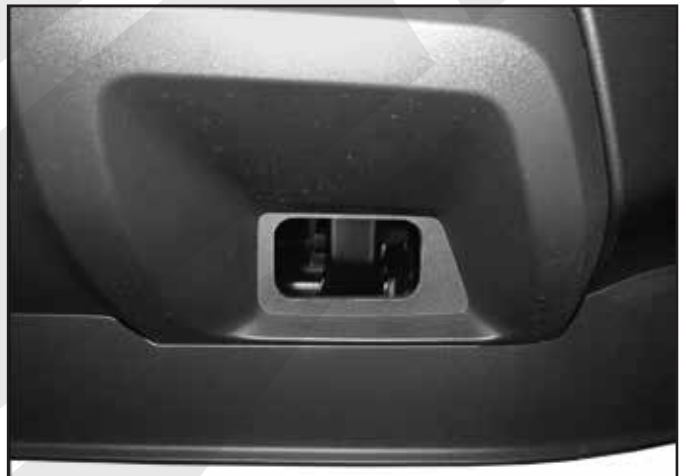
Bracket & Seal Removed
