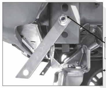
12mm x 35mm Bolt Plates 12mm Lock Washers 12mm Flat Washers 12mm Hex Nuts
