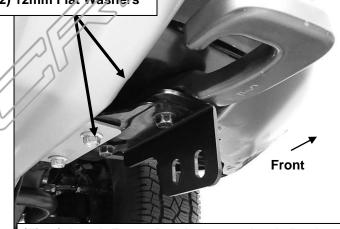
(Fig 2) Attach Frame Bracket to tow hook. Replace hardware with supplied longer 12mm Fine Thread Hex Bolts, Lock Washers and Flat Washers.
