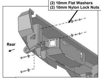
(Fig 13) Attach Bumper directly to integrated hitch bracket (see Fig 12)
