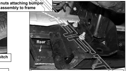
(Fig 3B) Remove the factory hex nuts attaching bumper assembly to frame. STD tow package model pictured (no receiver hitch)
