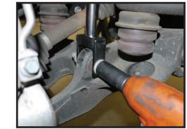
12. Route the remote reservoir forward by rotating the manifold in the proper direction.
