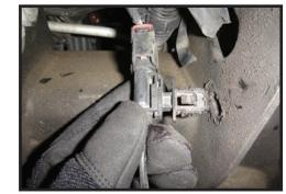
7. The supplied (250002) reservoir bracket will be installed into the large hole where the ABS clip was removed. Use the supplied (150014) nut tab and 3/8" bolt to fasten the reservoir bracket to the bucket as shown. [Torque to 45 ft-lbs] [FIGURE 2 & 3]
