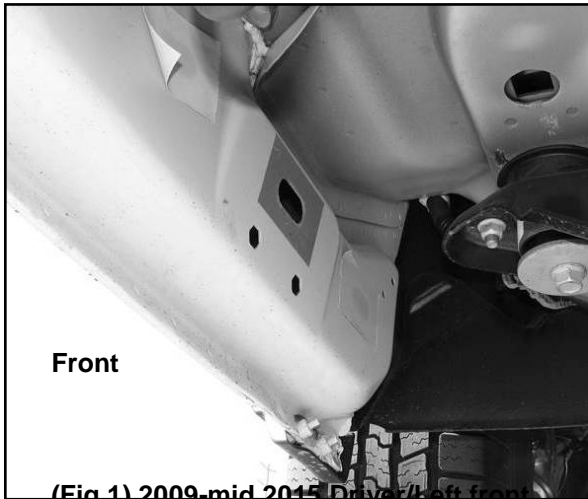
(Fig 1) 2009-mid 2015 Driver/Left front mounting location (No factory holes in pinch weld 2009-2012 models)
