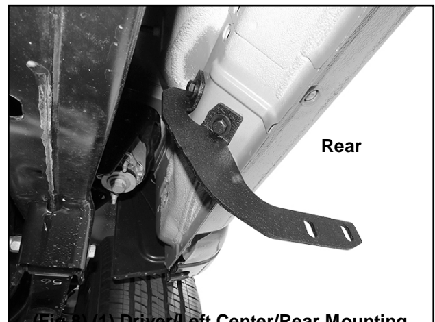
(Fig 8) (1) Driver/Left Center/Rear Mounting Bracket attached to the rear location
