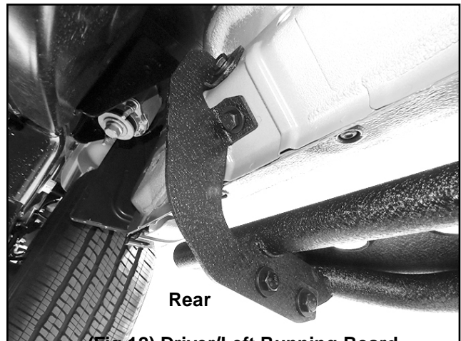
(Fig 12) Driver/Left Running Board attached to the rear location
