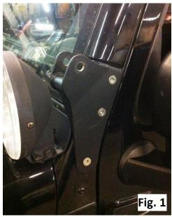
the assembled passenger side bracket against the side of the frame where the factory bumper mount holes are located. The pinch seam of the Jeep tub should set between the bracket and the clamp. Utilizing a factory bumper side bolt, loosely thread one through the bottom hole of the bracket into the frame. This is to hold the brackets into place while you slide the rear bumper back on. Repeat steps for the driver side. (Fig. 3)
