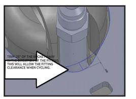
9. Once the shock bucket has been trimmed, install the coilover assembly by guiding the remote reservoir through the hole in the bucket and route the reservoir towards the front of the chassis.
