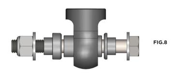
12. Reinstall the outer tie rod end. [Torque to 54 ft-lbs] Install cotter pin.
