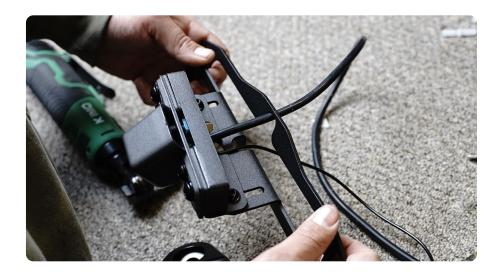
STEP 21 | Align the upper bracket so that it is straight and even, then secure the M6 hardware using a 4mm allen bit.
