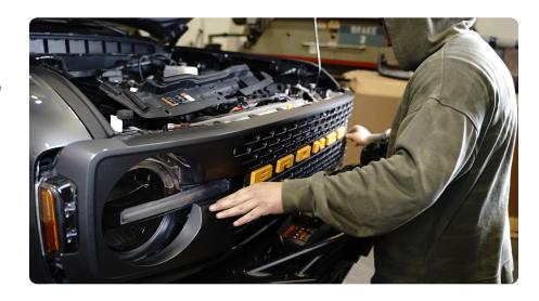
STEP 28 | Use a 13mm socket and the factory hardware to secure the grille to the vehicle.
