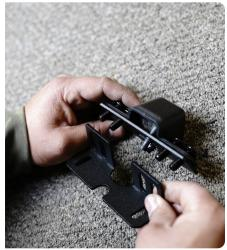
STEP 16 | Place the mount cover over it, and loosely secure with the provided M8 hardware.
