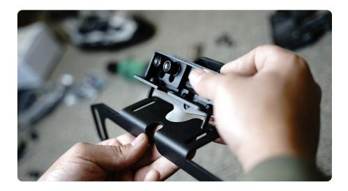
STEP 18 | Align the camera assembly and brackets so that the camera is sitting straight and even on the bracket.
