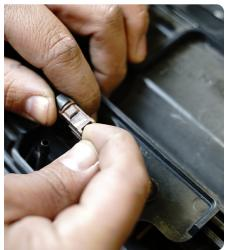
STEP 10 | Use a trim clip tool to remove the clips securing the camera hose to the grille and place it off to the side.
