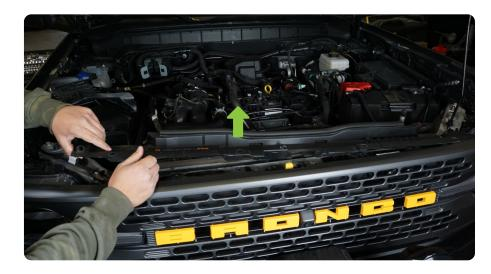
STEP 4 | Disconnect the camera wiring connector by pressing the release tab and pulling.
