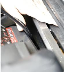
STEP 25 | For our install we routed under the grille, behind the passenger side headlight.
