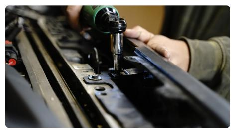
STEP 29 | Place the plastic grille trim back into place above the grille and pull the factory air intake cowl. Secure using the factory plastic grille trim using the factory push clips.
