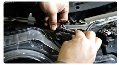
STEP 5 | If your vehicle is equpped with adaptive cruise control, disconnect it now by pressing the release tab and gently pulling on the connector.
