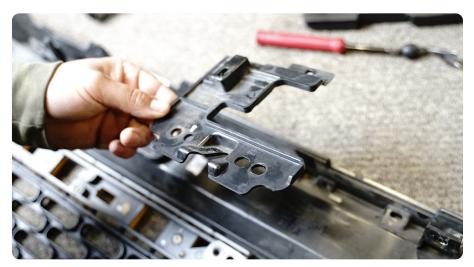
STEP 14 | You can now remove the camera housing assembly.
