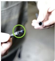
STEP 26 | Connect the camera wiring harness by pressing it into place until the clip is secure.
