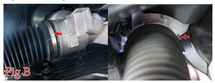
4. Push back the white plastic ring around the outer edge of the inner tie rod end, then use a crescent wrench to spin the inner tie rod off of your steering rack. Once the inner tie rod is removed, slide the plastic ring off of the steering rack shaft. (Fig C)
