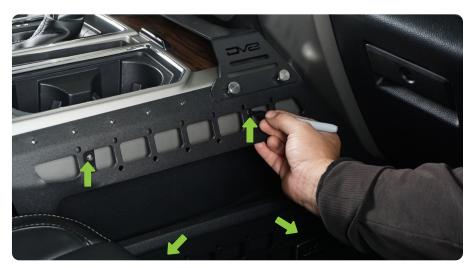
STEP 3 Using a 11/32 drill bit, drill the (4) mounting holes on each side.
