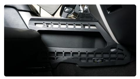
STEP 6 Using the (4) Locking Knobs, secure the Bridge piece to the side panels.
