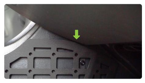
**STEP 6** Verify the bridge can be adjusted to sit evenly between the transmission shifter and transfer case shifter.
