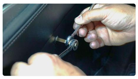
STEP 19 Use a 12mm wrench to hold the spacer while tightening with a 10mm socket. Tighten slowly until the nutsert is set properly. Do not over tighten.
