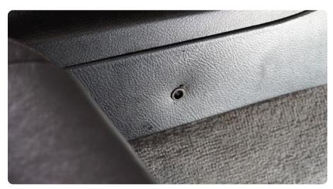
**STEP 10** | Disassemble the bridge and side panels using a 4mm allen bit.
