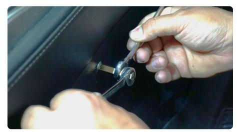
STEP 13 Use a 12mm wrench to hold the spacer while tightening with a 10mm socket. Tighten slowly until the nutsert is set properly. Do not over tighten.
