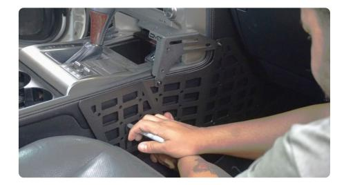
STEP 4 | Remove the assembly from the vehicle, and drill out the marked mounting holes with an 11/32" drill bit.
