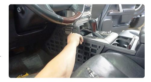
STEP 7 Use the provided nutserts and nutsert tool to install the nutserts into the mounting holes.
