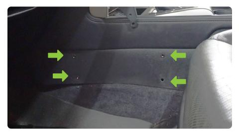
STEP 8 | Place the assembly back in the vehicle, and secure the passenger and driver side mounting hardware using the provided M6 hardware with a 4mm allen bit.
