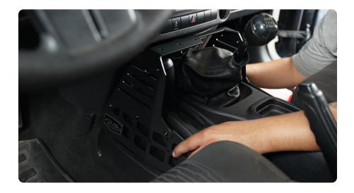
STEP 3 | With assistance, hold the assembly in the desired mounting location and mark the (4) mounting holes on each side of the assembly.
