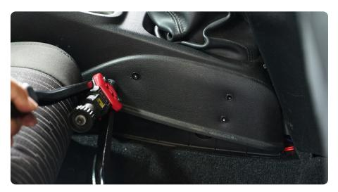
STEP 7 | Secure driver-side center console panel using a 3mm Allen bit or wrench and provided M5 hardware.
