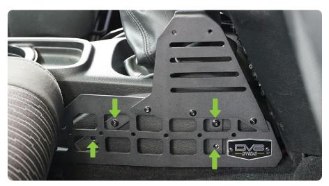
STEP 9 | Secure the driver-side panel to the center console bridge using a 3mm Allen bit or wrench and the provided M5 hardware.
