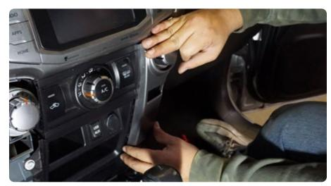
STEP 12 | Reconnect the wiring harnesses to the center console.
