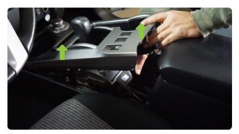
STEP 3 | Disconnect the two wiring harnesses under the center console by pressing on the release clips.
