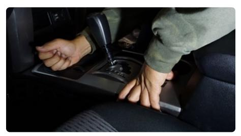
STEP 13 | Install the bridge using the provided M6 hardware with a 4mm allen bit.
