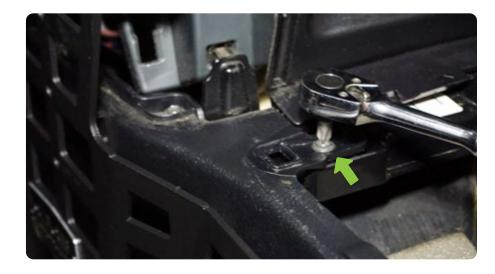
STEP 11 | Install trim pieces on the dash by applying pressure until the clips are secure.
