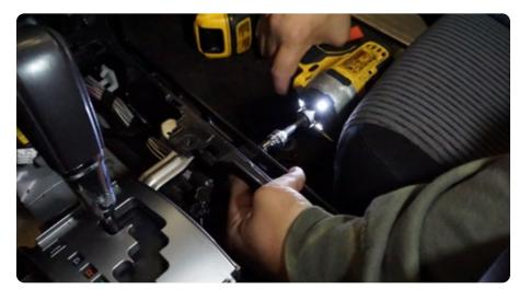
STEP 9 | Install factory bolts on both sides of transmission shift knob using a 10mm wrench and the factory hardware.
