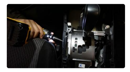
STEP 8 | Install both mounts using the provided M6 hardware with a 4mm allen bit. Reach back and apply pressure on the nut with your hand until "catches" and is secure. Use a 10mm wrench if necessary.
