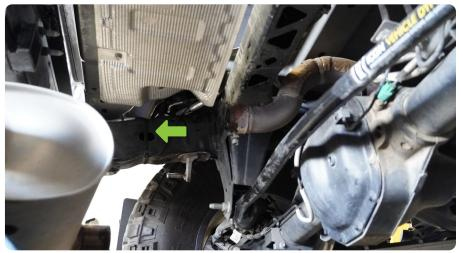
STEP 11 Use a 10mm socket and a trim clip tool to remove the factory hardware and plastic clip retainers securing the factory heat shield in place.
