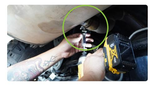
STEP 20 | Install the factory tiedowns using a 10mm socket and the factory hardware.
