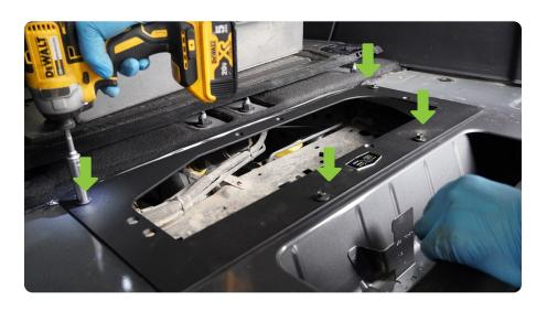
**STEP 13** | Place the DV8 storage box under the vehicle and lift it to the mounting plate by reaching down through the empty space in the cab.
