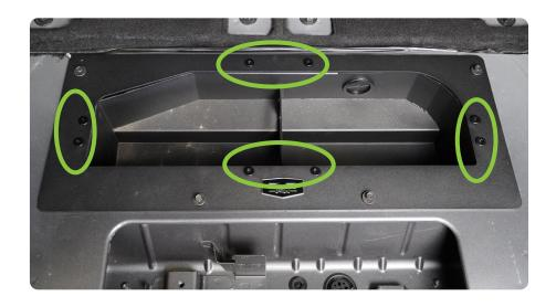
**STEP 15** | If you are mounting a compressor, do so at this time using the hardware provided with the compressor.
