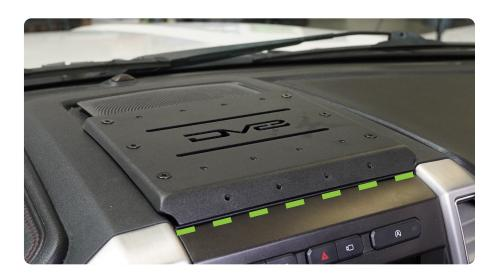
STEP 5 Remove the Dash Mount top by removing the (6) M6 screws using a 4mm Allen bit.
