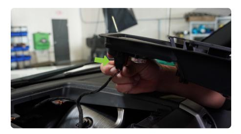
STEP 10 | With the factory dash pocket removed and the DV8 Dash Mount double sided in place, use a marker to mark the 4 holes you will need to drill into the factory dash pocket.
