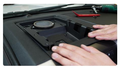
STEP 14 | Use a 7mm socket to secure the dash speaker using the factory hardware.
