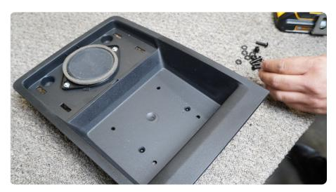
STEP 12 | Using a 4mm allen bit, 10mm wrench and provided M6 hardware, install the DV8 Dash Mount.
