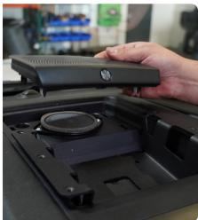
STEP 7 Using a 7mm Socket, remove the two bolts holding the dash pocket in place.
