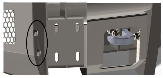
Figure 10a (bolt location for lower guard)
