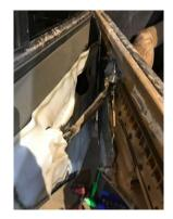
UNHOOK DOOR LATCH LINKAGE AND UNPLUG WIRES.
