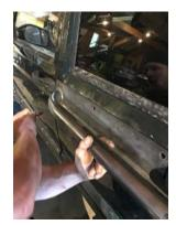
4. HOLD PANEL IN PLACE AND MARK HOLES WITH MARKER
