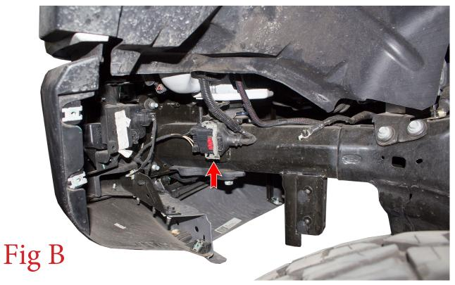
3. Using an 18mm Socket, remove the 3 bumper mounting nuts (per side). Then, remove the OEM Bumper from the vehicle. (Fig C)
