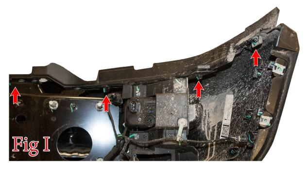
10. Remove the fog light assembly. Use a T40 Torx Socket to remove the top two bolts. Use a 10mm Socket to remove the bottom/sideways facing bolt. Use an 8mm Socket to remove the bottom nut. (Fig J)
