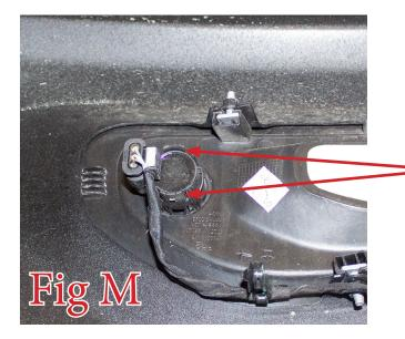
Spread these two tabs to release the sensor. Then, squeeze the tabs together to release the sensor mounting ring from the bumper.
