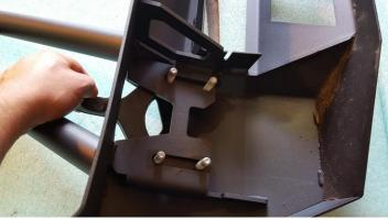
Figure 4: Installing OEM tow hooks
