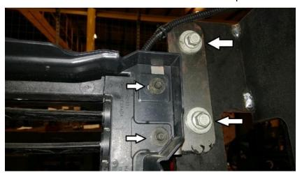
15. Install the fog lights to the light brackets by using the 3/8" carriage bolts and flange nuts. The light bracket will be mounted to the frontend using ½" carriages bolts, washers, and nuts.
