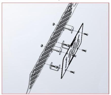
19. If the vehicle does not have a camera, install small insert by using the black button head bolts and nuts.
