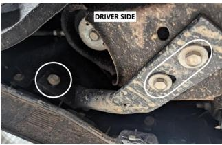
2. Remove the tow hooks by removing the two 18mm bolts. Two on each side. This will allow to reach the bottom bumper bolts. You will need to use a 18mm wrench or ratchet wrench(preferred).
