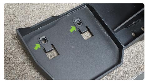
STEP 16 | Use the provide M12 hardware, a 21mm socket and 22mm wrench to secure bumper mounting brackets to the bumper.
