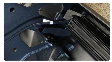
STEP 13 | If you are planning to run a winch, install the winch onto the provided winch plate using the hardware provided with the winch.
