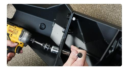
STEP 12 | If you are planning to run a light bar install the light bar now using the provided M6 hardware, light-bar brackets and hardware provided with the light-bar.
