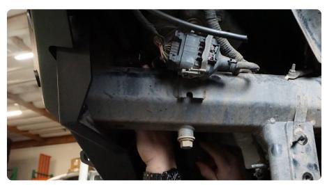
STEP 21 | Reconnect the bumper wiring harness to the vehicles main wiring harness and lock it in place.
