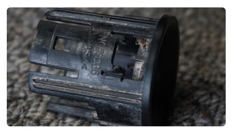
STEP 18 | Install the factory sensor bezel into the DV8 Front Bumper in the same order they were removed.
