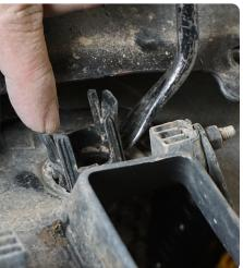
STEP 10 | Use a trim pry tool to remove the bumper wiring harness.
