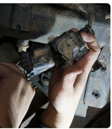
STEP 3 | Using a 18mm socket/ wrench, remove the six bumper mounting bolts (3 on each side).
