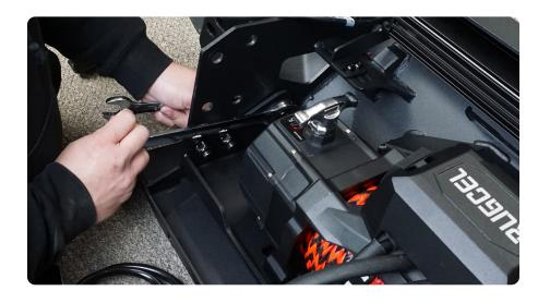
$\begin{array}{c|c} \text{STEP 15} & \text{Install provided Nut-clips} \\ \text{on to the bumper mounting brackets.} \end{array}$
