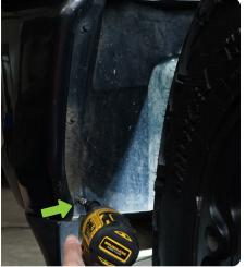
STEP 2 | Disconnect the bumper wiring harness.
