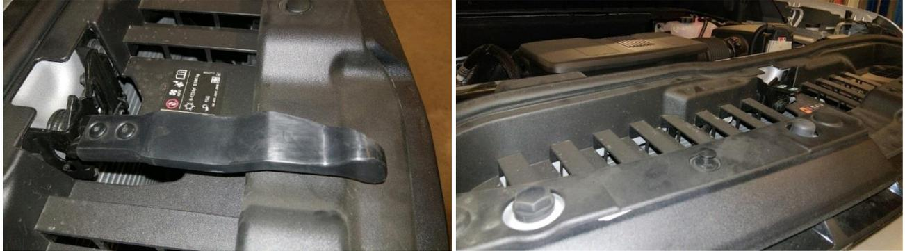
9. Disconnect the sensor/fog light wiring harness. Also, if vehicle is installed with a front camera, unhook the connector. The grille can then be removed by remove (4) 10mm bolts on top and pulling the grille away from the truck to release the clips.
