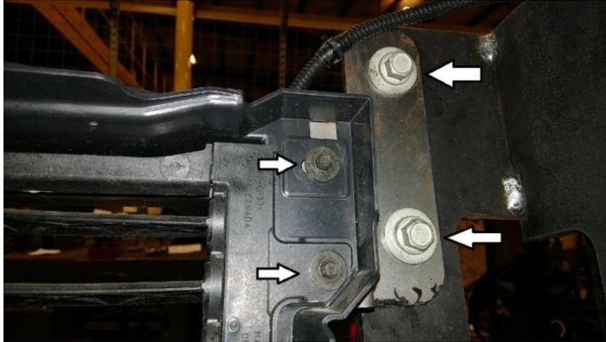
19. Mount the bottom brackets to the tow hook holes. Remove the tow hook bolts and use the 5" x 1/2" bolts to install. Use the 1/2" black carriage bolts to mount the frontend to the bottom brackets.
