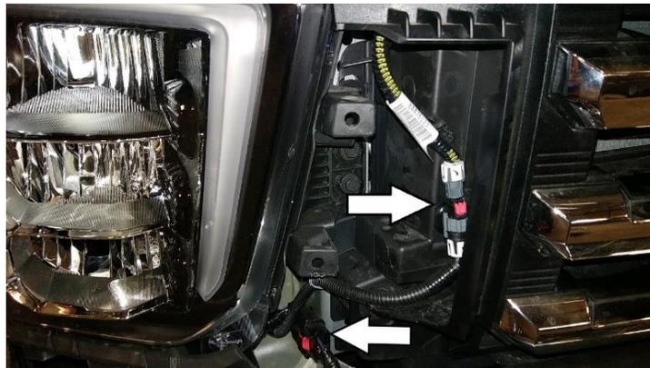
10. On vehicles with diesel motors, unplug the block heater plug.
