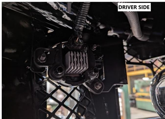
25. If the vehicle does not have a camera, install small insert by using the ¼” black button head bolts and nuts.
