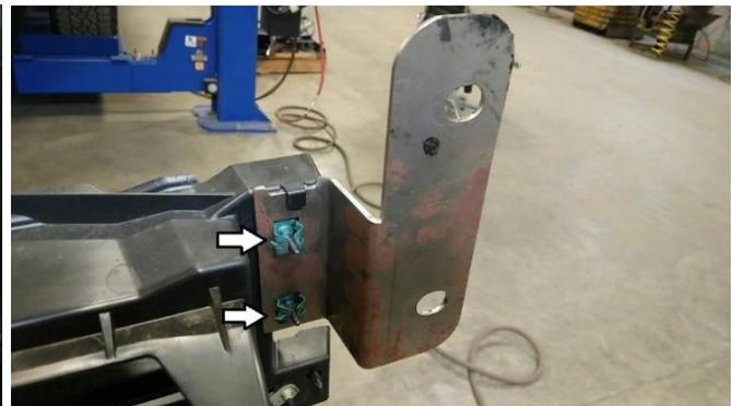
16. Remove the two black bumper mounting plate by removing the (4) 15mm bolts. The bolts will be used to install the Ranch Hand Frontend.
