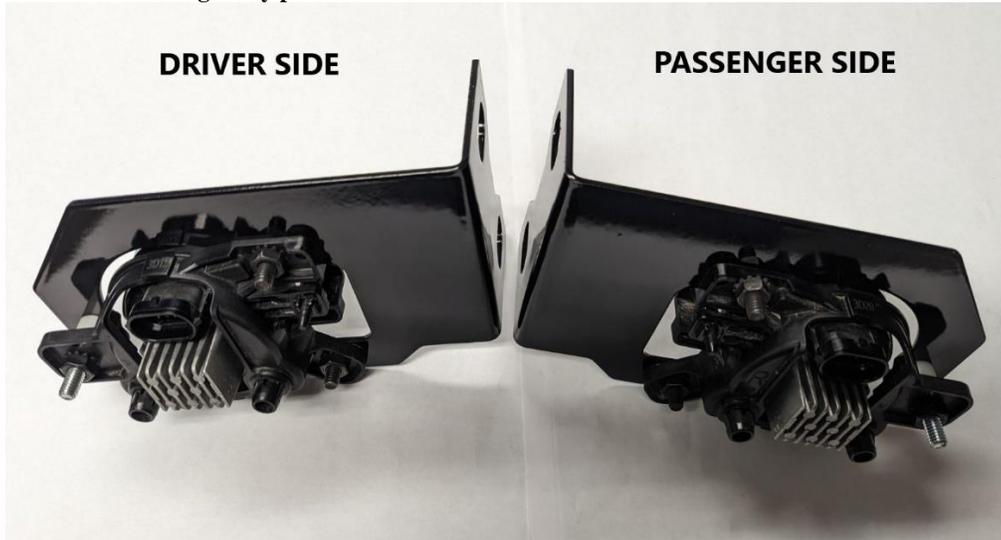
24. Mount the fog light/light bracket to the two lower holes of the upright. Use two ½” carriage bolts to install.
