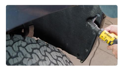
**STEP 30** Using a T15 Torx bit, install the upper grille bolts.
