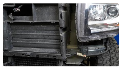
**STEP 16** | Remove the active grille shutters using a 10mm socket.
