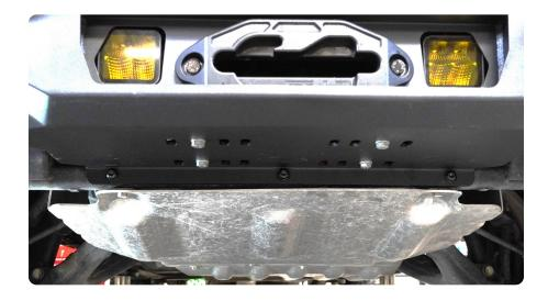
STEP 27 | Once bumper is secure, install front bumper fascia onto truck in reverse from when it was removed. Ensure to watch the sides to prevent damage to the fenders.
