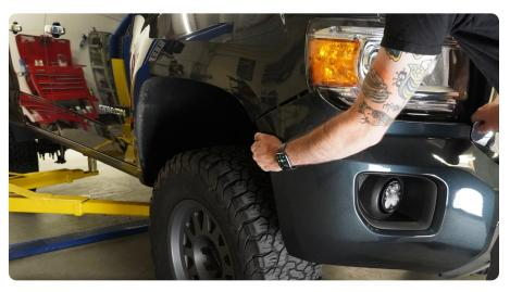
STEP 28 | Reinstall the (3) 7mm bolts on each fender flare.
