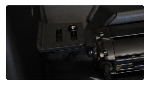
STEP 22 | If running 3" pod lights, install now. Mount using hardware provided with the light.
