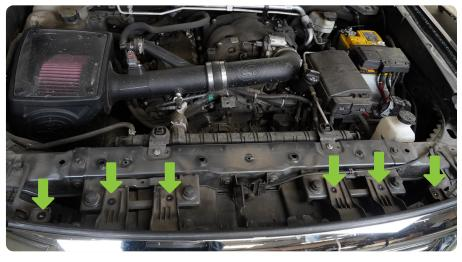
STEP 31 | Using your factory push pins, install the radiator support cover.
