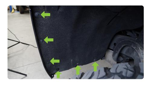
**STEP 4** Fold back the inner fender to gain access to back of the factory front bumper.
