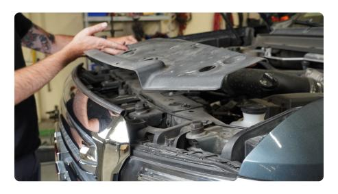
STEP 2 | Use a T15 Torx tool to remove the (6) bolts retaining the front grille.
