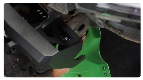
STEP 25 After the Dv8 bumper is installed using the (4) crash bar bolts, (if equipped with the factory skid plate) using a 16mm socket, remove the front (2) bolts and loosen the rear (2) bolts to lower the skid plate.
