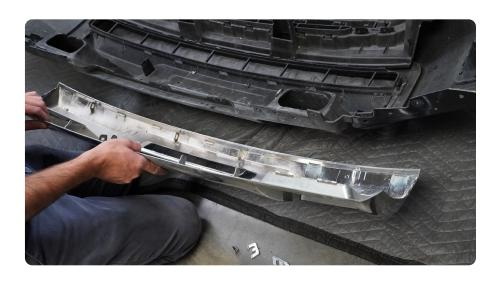
STEP 14 | Once removed, cut out center portion of the plastic as shown.
