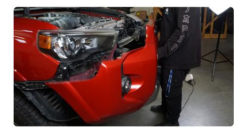
STEP 11 | Disconnect the bumper wiring harness. To disconnect, rotate the white locking tab and then pull to remove.
