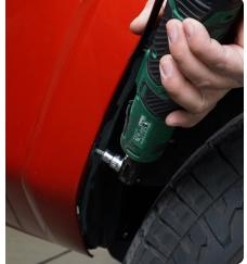
STEP 6 | Use a 10mm socket to remove the center bolt along the bottom of the grille/valance.
