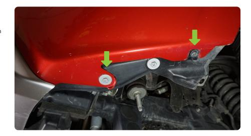
STEP 8 | Gently pull the inner fender to release the clips securing it to the vehicle.
