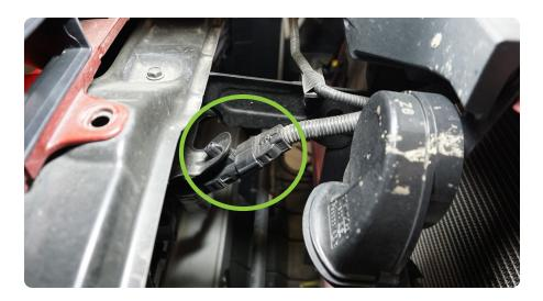
$\begin{array}{c|c} \textbf{STEP 35} & \textbf{Re-install the factory trim} \\ \textbf{clips securing the grille to the vehicle.} \end{array}$
