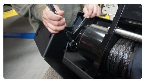
STEP 27 | With assistance, lift the bumper to the vehicle and secure it to the vehicle using the factory hardware with a 14mm socket.
