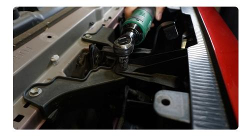
STEP 37 | Re-install the remaining trim clips securing the valance to the grille.
