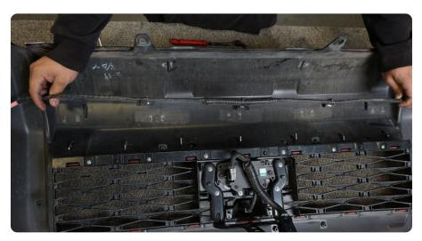
STEP 15 | Use a trim clip tool or flathead screwdriver to remove the plastic fasteners securing the valance to the bumper.
