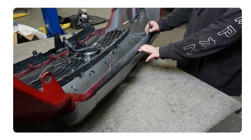
STEP 17 | Move and secure the wiring out of the way to prepare to trim the bumper.
