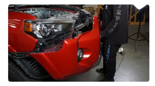
STEP 29 | Secure the grille/bumper to the vehicle using the factory hardware with a 10mm socket and extension.
