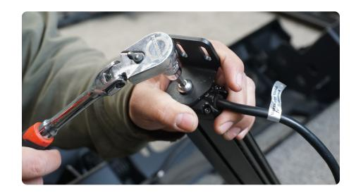
STEP 24 | When securing the brackets for the light bar, be sure the light is centered and even before securing.
