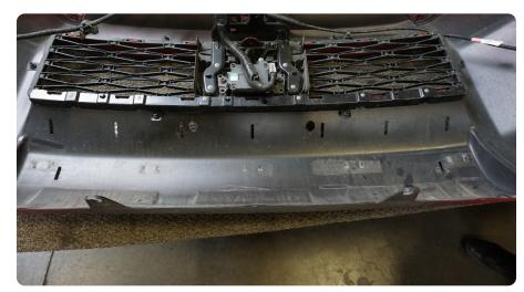
STEP 18 | Remove the grille from the bumper by using a trim clip tool or flat head screwdriver to gently pull back the tabs securing the grille.
