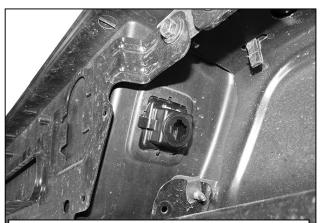
(Fig 5) Disassemble bumper to remove license plate lights, trailer plug, sensors and wiring harness from bumper as equipped
