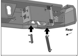
(Fig 12) Insert "Short" and "Long" 10mm Double Bolt Plates into back of Bumper. Use 10mm Plastic Retainers to hold Bolt Plates in position (retainer use optional) **WARNING!** Do not crawl under bumper unless the bumper is properly supported on blocks or stands or the bumper may fall.
