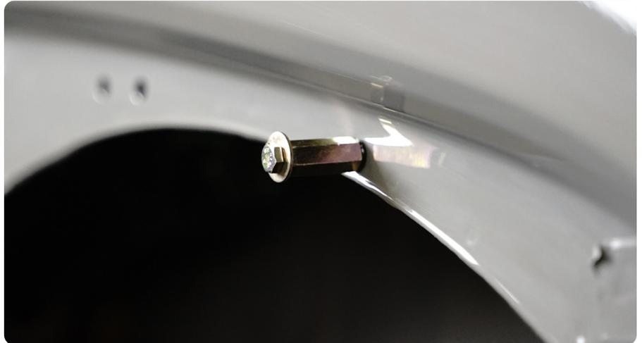
**STEP 18** | Use a 12mm wrench to hold the spacer while tightening with a 10mm socket. Tighten slowly until the nutsert is set properly. Do not over tighten.
