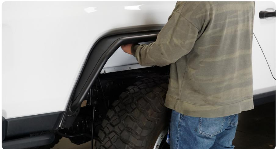
**STEP 13** | Install the fender flare onto the vehicle using the provided M8 hardware with a 5mm allen bit (and 13mm wrench if using nuts).
