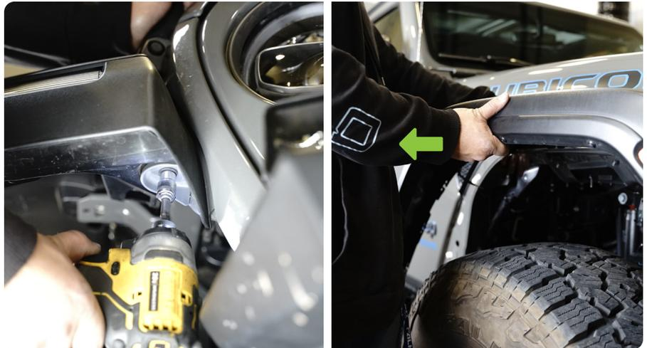
**STEP 4 |** Use a trim clip tool to remove the factory clips along the fender.
