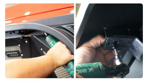
STEP 11 | Route and secure the wiring to your preference and install the new turn signal into the factory connector.
