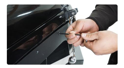
STEP 11 | Route and secure the wiring according to preference and install the new signal into the factory connector.
