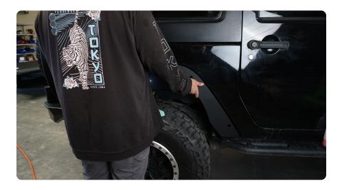
STEP 14 | Install the fender flare onto the vehicle using the provided M6 hardware with a 4mm allen bit.
