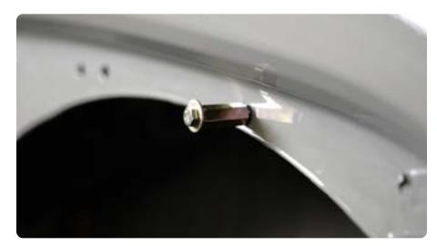
STEP 19 | Use a 13mm wrench to hold the spacer while tightening with a 10mm socket. Tighten slowly until the nutsert is set properly. Do not over tighten.
