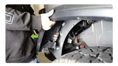
STEP 7 | Use a trim clip tool to remove the clips along the edge of the fender.
