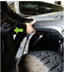
STEP 4 Use a trim clip tool to remove the factory clips along the fender.
