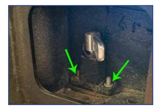
Shown in photo below is how it looks from underneath the arm. The center pin will need to be aligned with the drop pin plate from step 30 before tightening down the plate.
