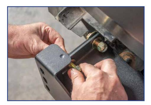
In this step, take another 1/2" washer and bolt and place it through the frame bracket and vehicle frame from the top (see below) and secure with provided nut retainer.
