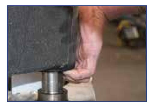
Grease the top bearings and place them onto the arm and onto the spindle. Again, you will likely need to wiggle the arm and swing back and forth so that the bearing is seated correctly and the arm looks level while opening and closing with ease.
