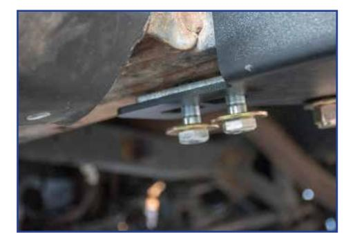
Now that we've secured the driver's side frame brackets, you'll repeat these steps for the passenger side. We recommend having an extra pair of hands to pull the exhaust pipe out of the way in order to get the additional bolts inserted from underneath.
