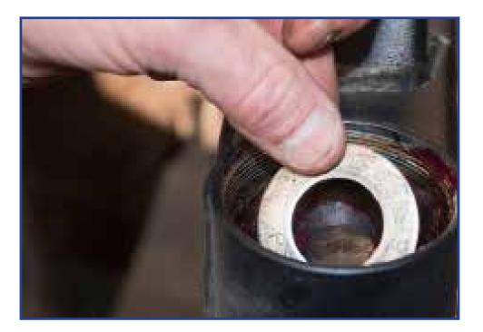
Next we'll drop the included large spindle nut and hand tighten onto the top of the spindle.
