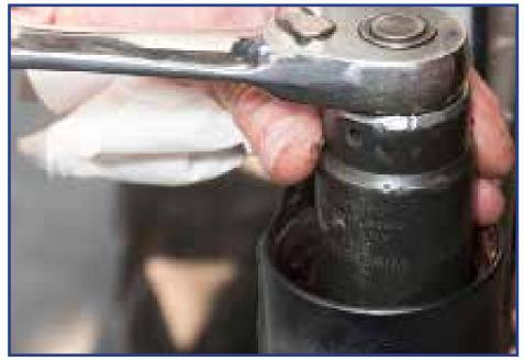
Use the included anti-seize packet and smear a decent amount along the threads of the top spindle cap.
