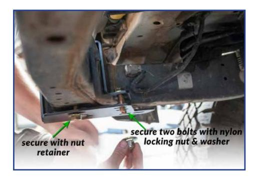
Take the included two-holed spacer provided in kit and place between the frame bracket and vehicle frame. (see photo below and step 7)
