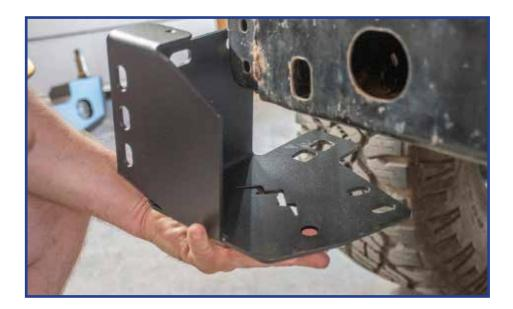
Attach the top frame mount bracket shown below over the vehicle frame and secure both with provided 1/2" bolts, washers and nylon locking nuts. (see step 3)
