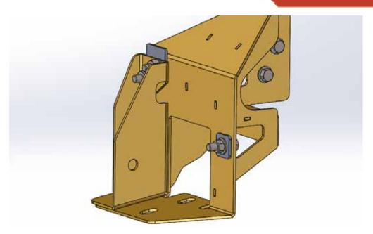
Use provided 1/2" bolts to attach your bumper onto the reinforcement brackets.
