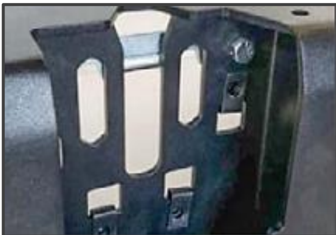
Welded Rod Plate should face inside the bumper and mounted in the upper most position
