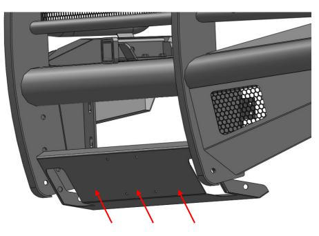
Figure 4 - Lower Guard Installation
