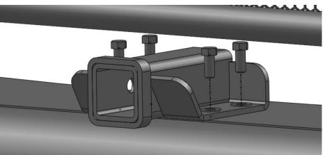
**Figure 6 - Hitch Installation**
