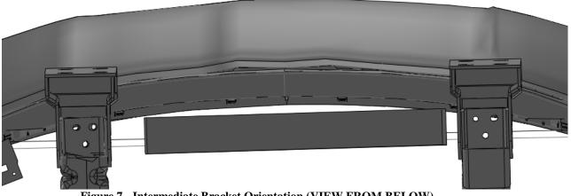
Figure 7 - Intermediate Bracket Orientation (VIEW FROM BELOW)
