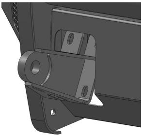
**Figure 5 - Shackle Bracket Installation**
