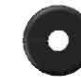
DETAIL C SCALE 1:1 NOTE: YOU'LL NEED TO MAKE A SLIT IN THE RUBBER GROMMET
